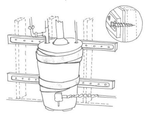
There should be very little space between the water heater tank and the wall. If there is more than one to two inches, attach a wooden block (for example, a 2 x 4) to the wall studs with long lag screws. The goal is to create a snug fit between the tank and the wall.
