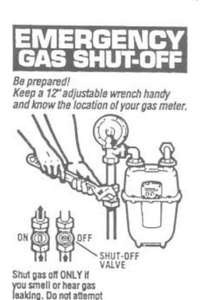
Shutting Off the Gas after an Earthquake
